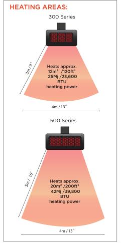
\*Heat area dependent on ambient temperature and wind. Optimum conditions experienced at approx 15.5°C/  $60^\circ\text{F}$  & low wind
